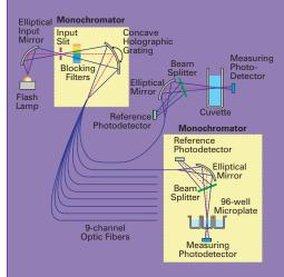
The SpectraMax Reader's optical system mimics a dual-beam spectrophotometer. Each sample has a discrete sample beam and reference beam.
