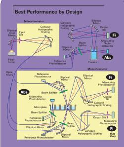
The design of the SpectraMax M2 Reader's optical system provides performance similar to a dedicated spectrofluorometer or spectrophotometer and is the only optical system that has integrated a dual-mode cuvette port and microplate reading.
