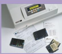
SpectraTest Validation Test Plates for absorbance and fluorescence intensity provide a complete traceable solution for validating optical performance of the SpectraMax M2 Reader, automatically.
